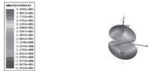
Figure 8: 3D Radiation pattern at 2.36GHz.
