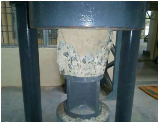
Fig. 2. Compressive Strength Test of Cube Specimen
