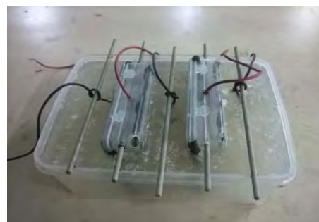
Fig. 2. Experimental setup of three chambered MFC-2 &amp; MFC-3
