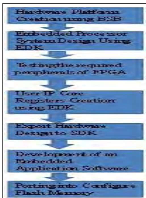
Fig. 3. Configuration of embedded system processor
