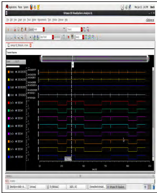
Fig. 9 Outputs y[0] to y[7] of 8 bit ALU
