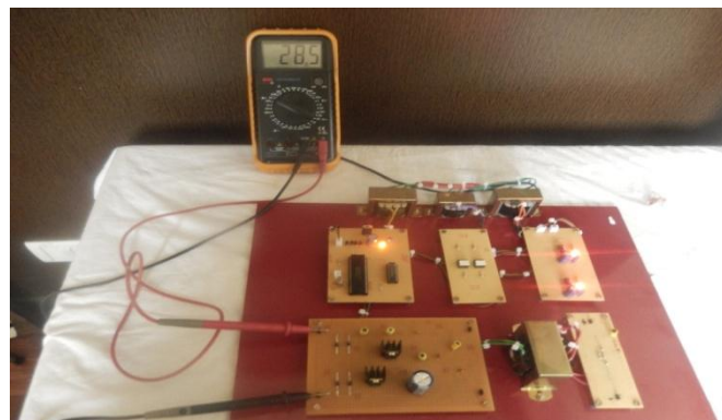
Fig. 21: Experimental Setup for Single Stage AC-AC Converter
