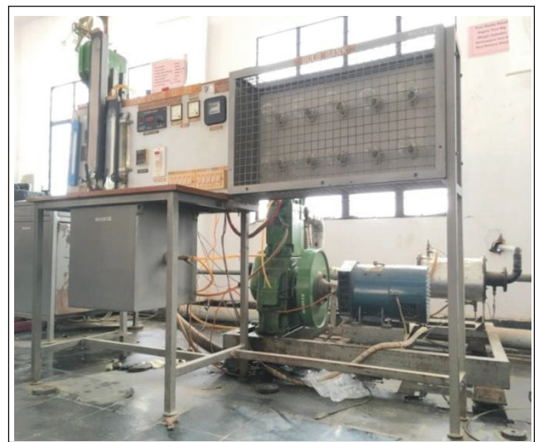
Fig. 1: The Engine Setup with an Alternator and Circuits (Courtesy: HKBKCE, EC Lab)
