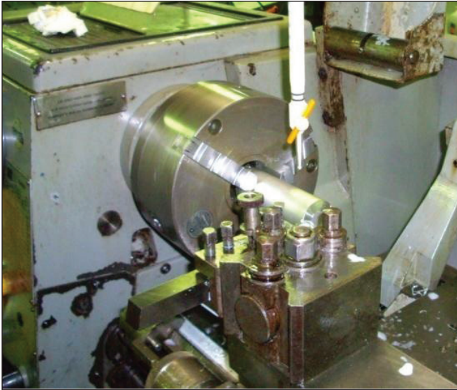
Fig. 1: Physical Orientation of Machining with MQL
