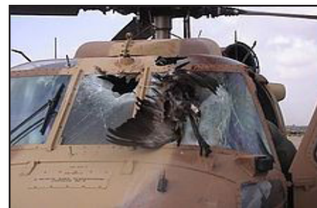
Fig. 1: UH-60 Black Sikorsky Hawk collision with a Bird Cause Damage to Windshield
