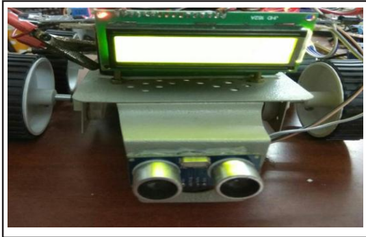
Fig. 9: ADSS Front View with Ultrasonic Sensor and LED Display to Detect the Vehicles in Front Direction
