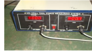
Fig. 3: Drill Tool Dynamometer
