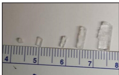
Fig. 4: Different Size of Transparent High-Quality Crystals Grew at pH=8 in the Solution. These Crystals were Harvested for Characterization
