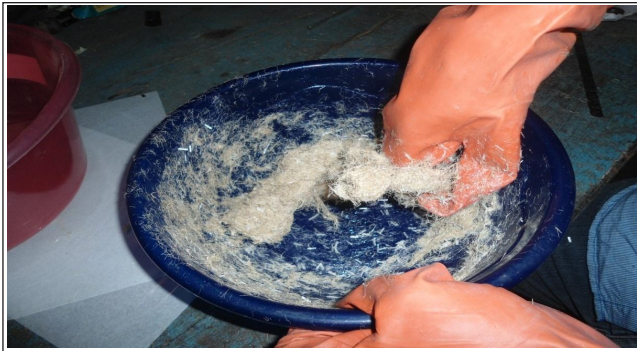
Fig. 5: Mixing of Resin and Palm Sprout Fiber
