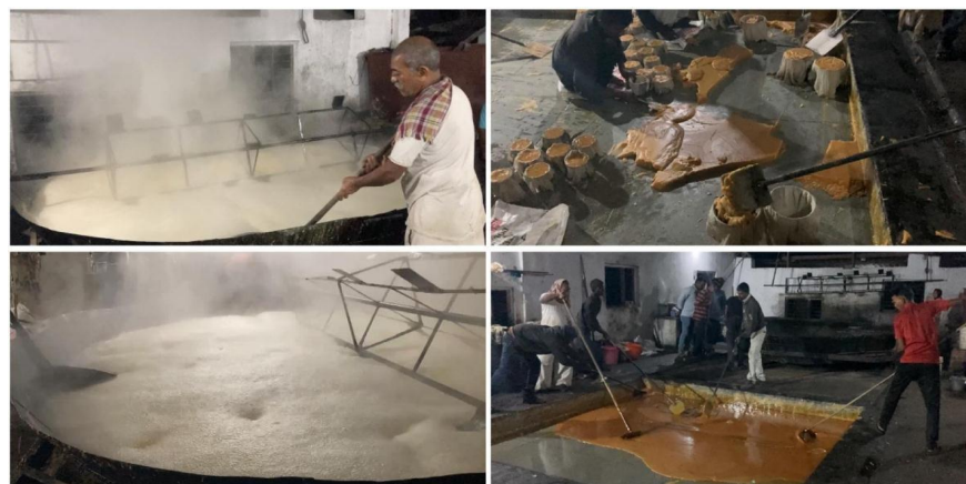
Fig. 2: Jaggery Concentration Process Done in a Traditional House of Mr. J. Jadhav, Local Jaggery Producer, Kagal (Kolhapur)
