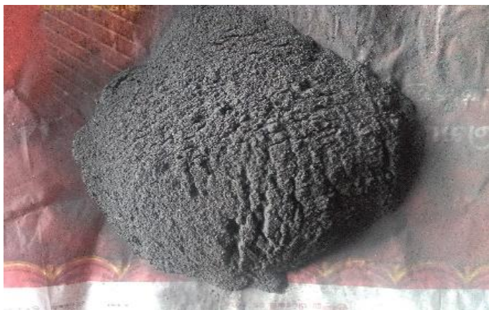
Fig. 1. Combination of Coconut Shell and Egg Shell Ash
