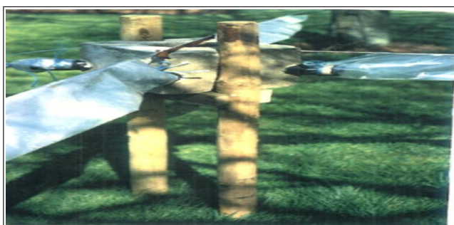
Fig. 7: The Block Supported by the Two Pieces of Timber Nailed to the Posts
