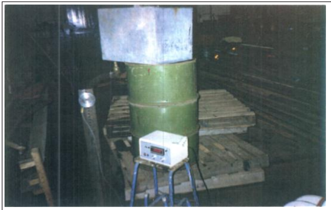
Fig. 3: The Load Cell and its Meter Together with the Water Supply Tank, Showing the Discharge Valve and Delivery Pipe
