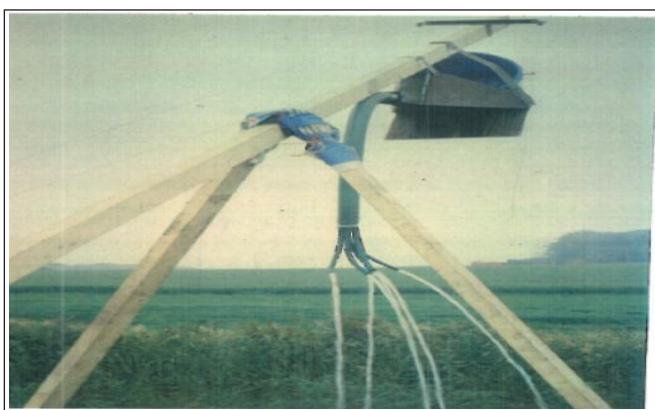
Fig. 8: The Flow Splitter Discharging Water at the Brook
