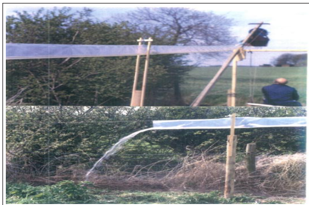
Fig. 6: The Polythene Envelope Directly Joined to the Single Bucket Lifter: Water Can be Seen Flowing Out of the End of the Envelope
