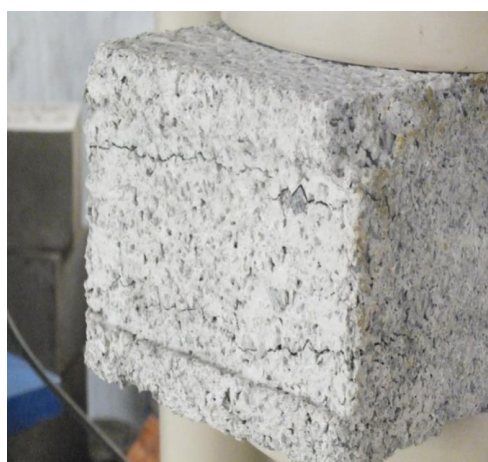
Figure 3. Compression test on hollow blocks
