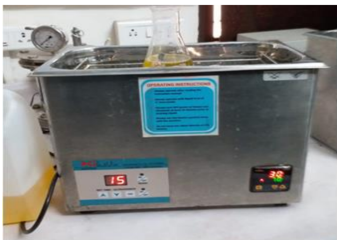
Figure.2: Mixing of solution in an ultrasonic homogenizer
