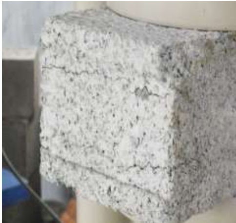
Figure 4. Compression test on hollow blocks
