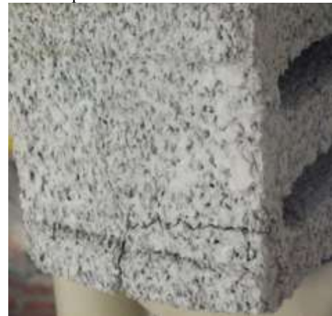
Figure 3. Compression test on hollow blocks
