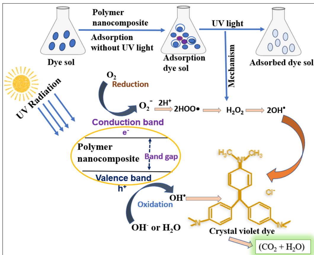
Fig. 5: Illustrative Diagram Depicting the Degradation of Dye using Polymer Nanocomposites
