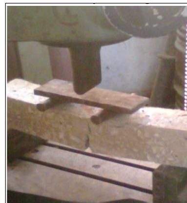
Fig. 6: Flexural Strength Test on Concrete Prism after 7 and 28 Days of Curing
